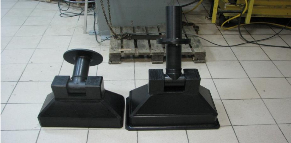
The prototypes no1 and 2 of the mouth body adjusted to different brush sizes
