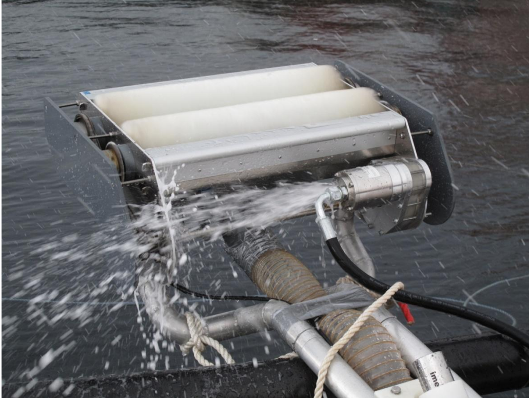
Netwash unit idling with the exoust water flowing out of the engine, and to the left. Camera visible down at the right side.
